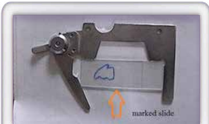
Fig. 1. The marked slide contains a hand-drawn mask of the landmarks on the parent slide. The use of this mask allows one to compare the same microscopic area from one slide to the same area from the same tissue block but that was stained with different stains on other slides.
