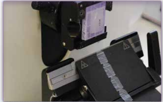
Fig. 3. A ribbon as it is being cut from the paraffin block, which contains many sections that will be separated into individual sections for storage. Black cardstock is taped to the microtome, providing support for the ribbon as it is cut while also offering good contrast to the white paraffin, making it easier to visualize the ribbon and its many sections.
