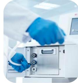
Color-coded drain and fill ports
