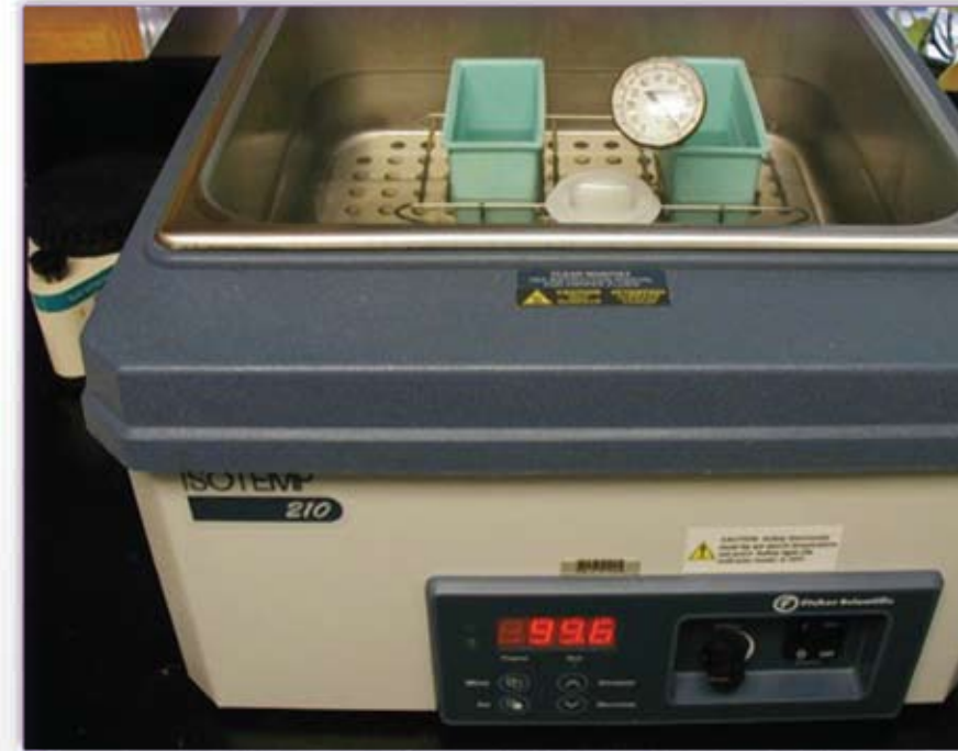
Fig. 2. Containers are placed inside the high temperature water bath to preheat the retrieval solutions prior to inserting the slides. Once the slides are placed, the lid is closed and the solution temperature is monitored with the dial thermometer. When the working temperature is reestablished, the timer is set for the desired length of the heating cycle. The water bath lid is open for demonstration purposes only and should remain closed throughout the procedure.
