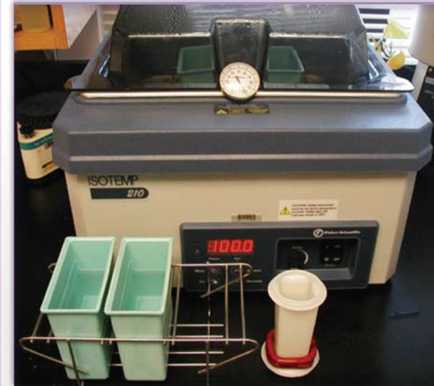
Fig. 1. Wire stain racks and vinyl-coated lead wire prevent the containers from tipping over. The water bath is used at 98°C -100°C. Temperatures are monitored with a dial thermometer.
