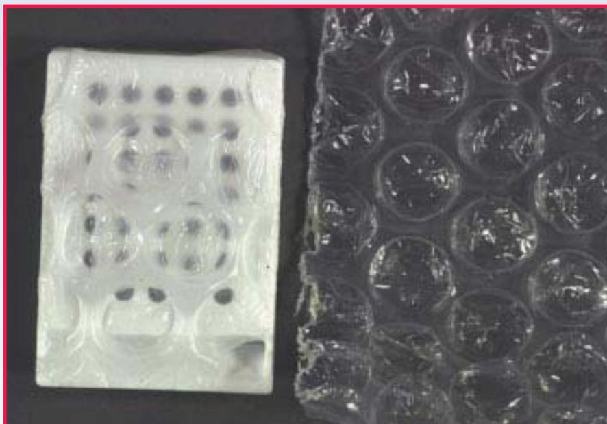
Fig. 1. The bubble wrap melted into the paraffin block, contributing to the loss of the specimen.
