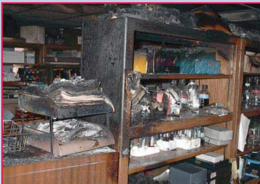
freezer leads one to believe that ignition was probably caused by the interior thermostat after the requisite accumulation of vapors. It was a big bang for such a small volume of liquid.
