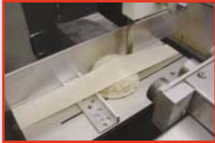
Fig. 2. Exakt Saw modifications that enabled uniform slab sections to be obtained.
