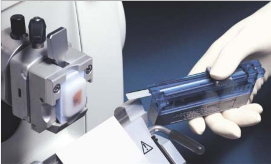
Meet two partners well-equipped for the high-volume demands of today's histology laboratory. Together, **Accu-Edge® Disposable Blades** and the **Accu-Cut® SRM™ 200 Rotary Microtome** – both from **Tissue-Tek®** – create the ideal sectioning system.
