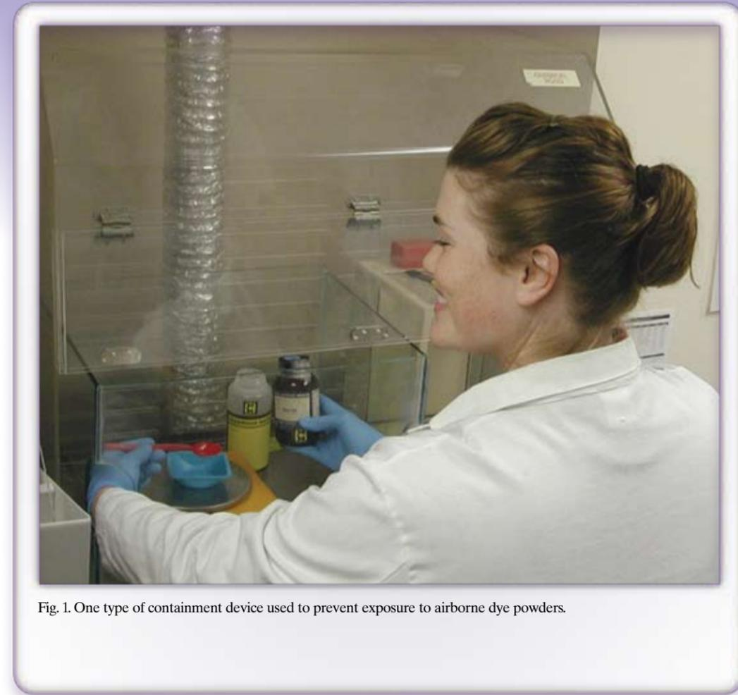
Fig. 1. One type of containment device used to prevent exposure to airborne dye powders.
