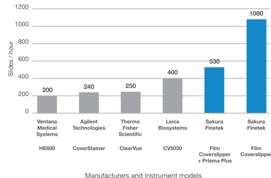
Throughput comparison of standalone coverslipppers and staining and coverslipping systems
